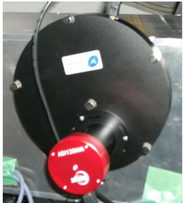
Fig.1. Filter-Wheel and WebCam
