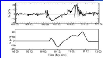
The temporal behavior of Bz at 1AU (the upper one is the observation by WIND and the other is simulated result)
