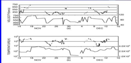
The predicted results(lower) compared with IMP8 observation(upper) The right ordinate stands for the values at 2.5 RS and the left ordinate for the values near the earth.
