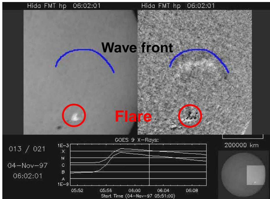
The FMT is quite effective to detect intersections of shock waves on the solar chromosphere (Moreton waves).
