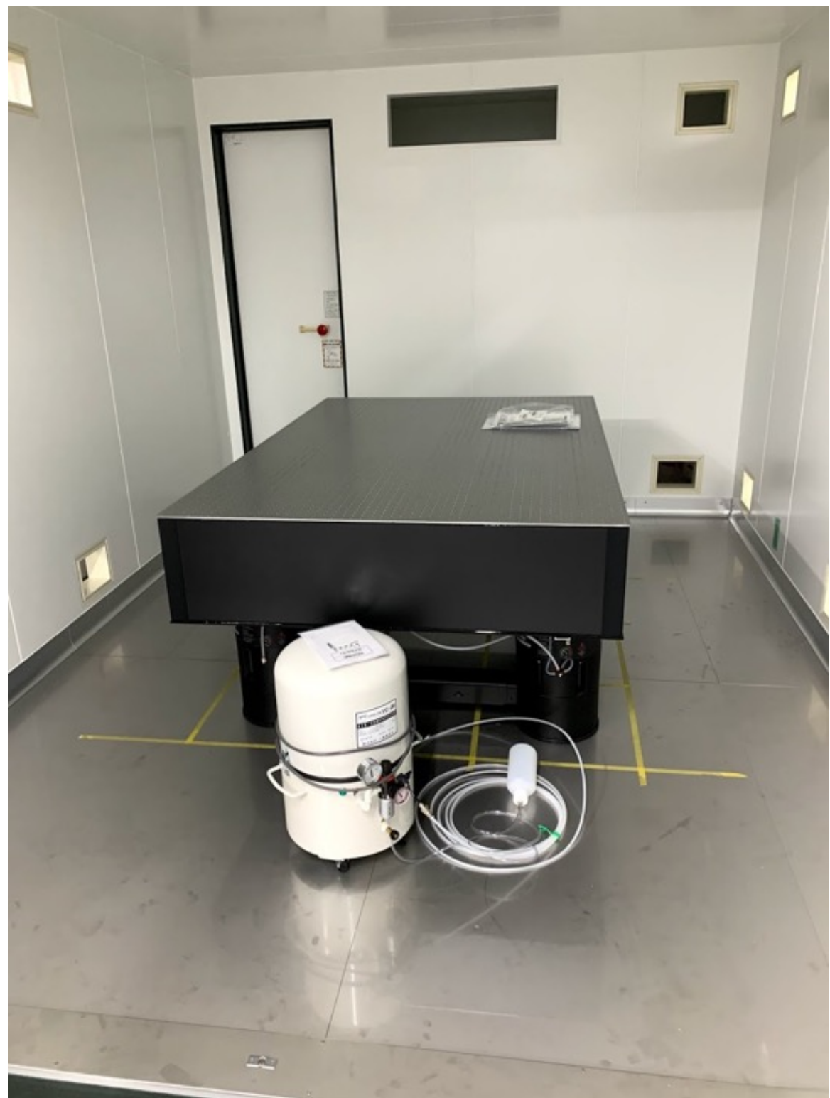
Newport製 RS2000 Series Optical Table 1200 x 1800 x 305 mm
