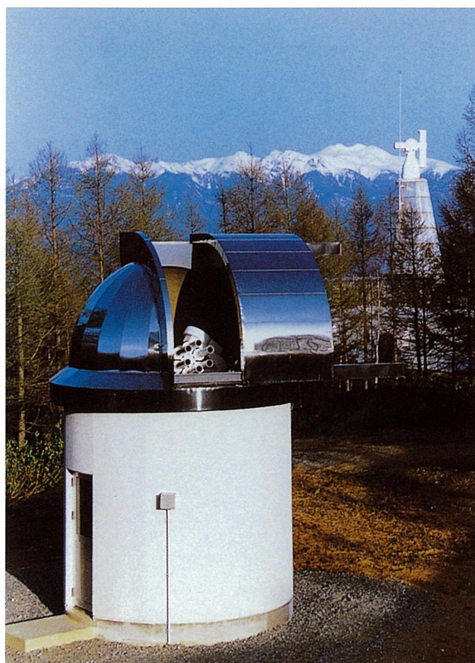
The Solar Flare Monitoring Telescope and its 3m dome
