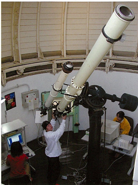
H \alpha monochromatic imaging system Sartorius 18cm refractor with a Lyot filter (band width: 0.5Å) and a CCD camera.
