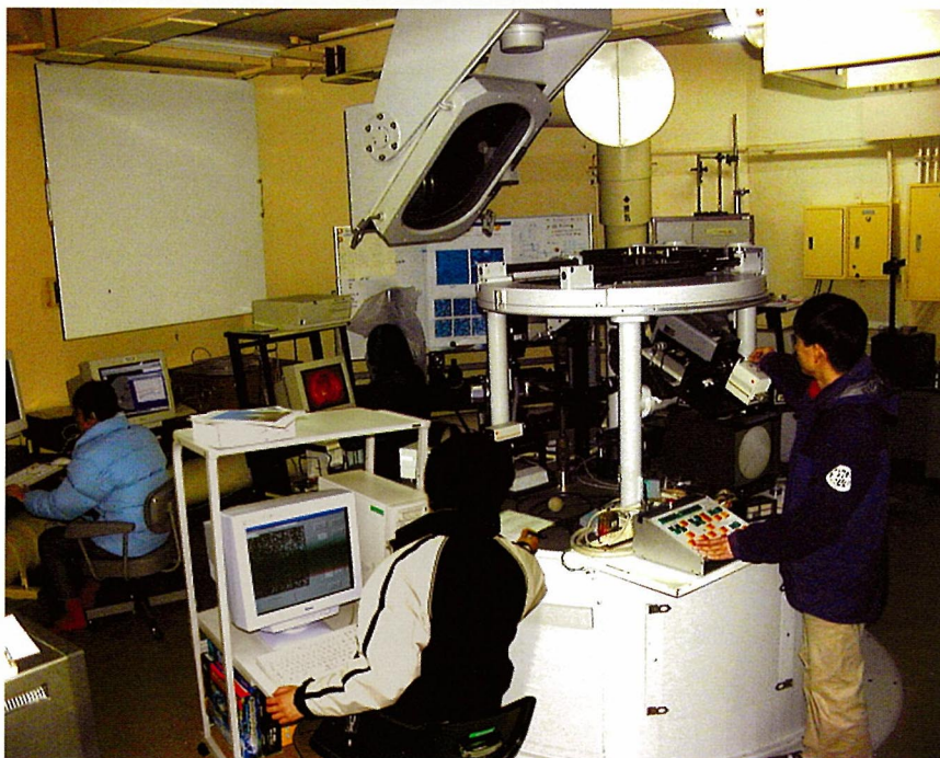
Observation with the high resolution vertical spectrograph which consists of an imaging unit and the spectrum observation unit.
