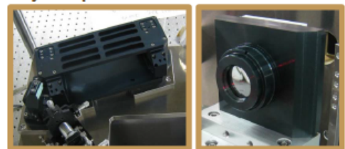
Slitjaw optics: mirror unit & filter unit
