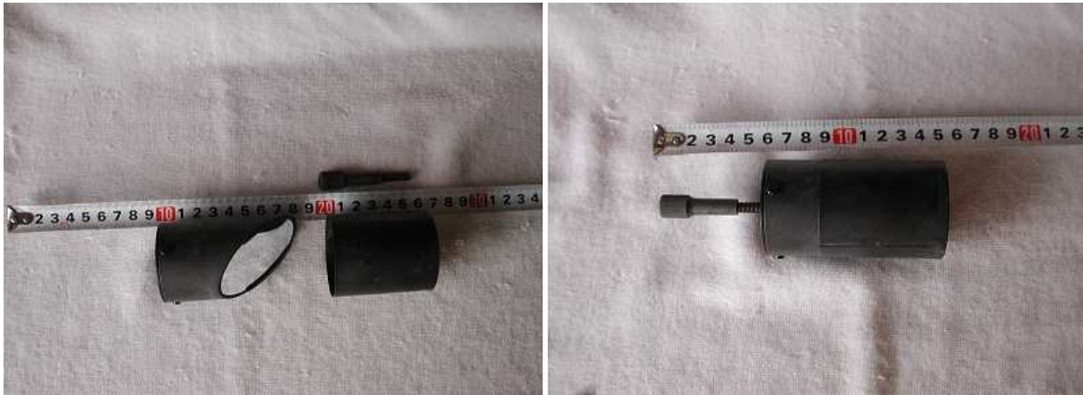
Secondary mirror (42×62mm Oval-shaped flat mirror by Takao Namura)
