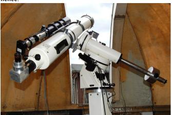
The instruments used:- 6inch Vixen that was stopped to 4.5", for the above images, showing a home made Herschel wedge in the picture, used for the 18ths white light shot of 0999, with full aperture yellow ERF 80mm TMB, Daystar ATM .6Å all on an AP 1200QMD. Best wishes
