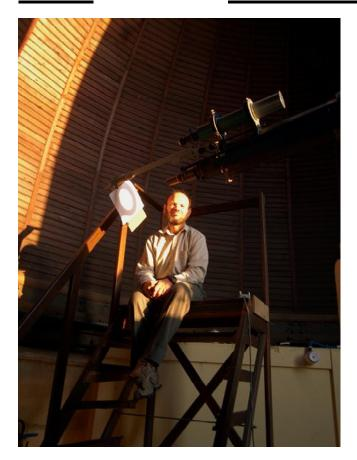
sharper than those of larger telescopes. Both the 7 ton bronze cupola and the instrument are moved by hand, except for small corrections with the right ascension motor, which also turns the instrument to compensate for the rotation of the earth.
