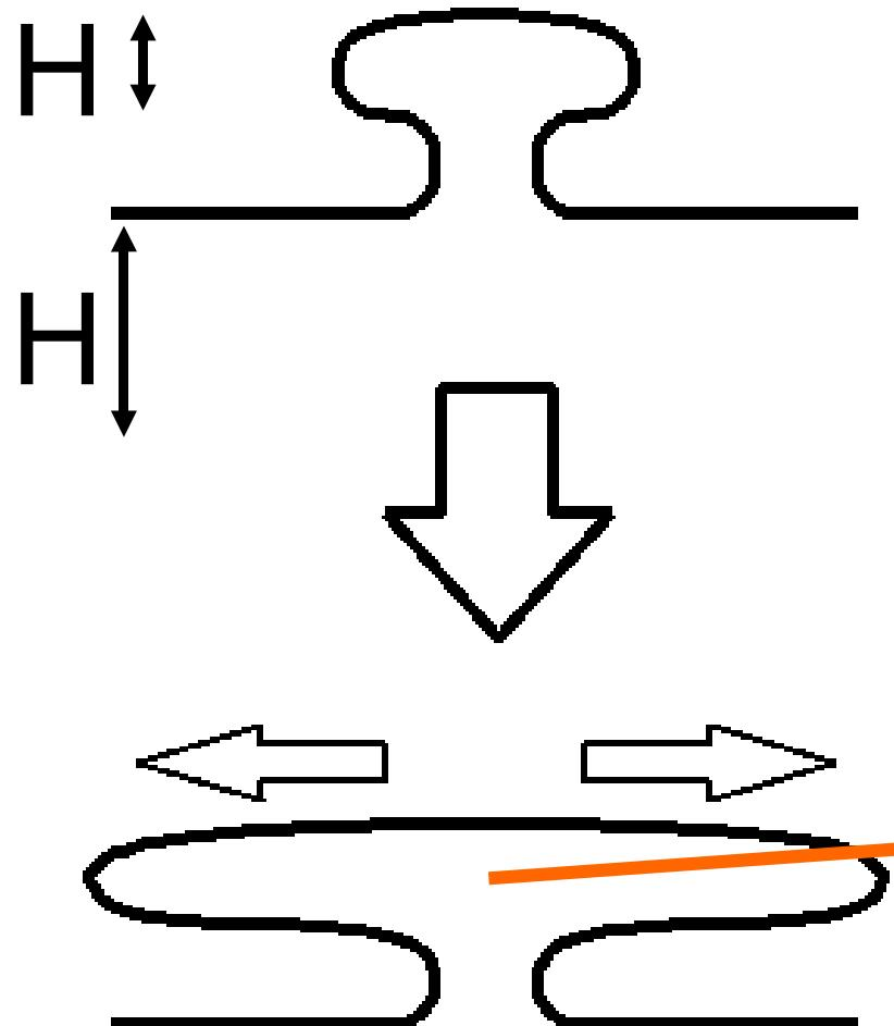
The magnetic flux expands horizontally until the magnetic pressure of the sheet is balanced with the surrounding gas pressure.
